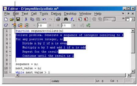
Commenting in Java and C/C++ Files Using the MATLAB Editor/Debugger. For Java and C/C++ files, selecting **Text** -> **Comment** adds the // symbols at the front of the
