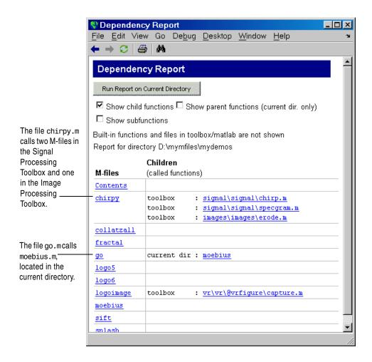
The Dependency Report is similar to running the depfun function, although the two do not provide the exact same results. For performance purposes, the Dependency Report limits the functions considered.
