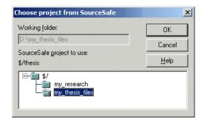
The selected file, its directory, and all files in the directory, are associated with the source control system project you selected. For the example, MATLAB associates all files in D:\my\_thesis\_files with the source control project my\_thesis\_files.
