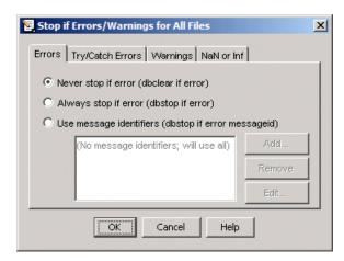
For example, to pause execution when a warning occurs, select the **Warnings** tab, and from it select **Always stop if warning**, then click **OK**. When you run an M-file and MATLAB produces a warning, execution pauses, MATLAB enters debug mode, and the file opens in the Editor/Debugger at the line that produced the warning. To remove the warning breakpoint, select **Never stop if warning** in the **Warnings** tab and click **OK**.
