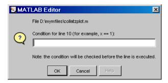
**2** Type a condition in the dialog box, where a condition is any legal MATLAB expression that returns a logical scalar value. Click **OK**. As noted in the dialog box, the condition is evaluated before running the line. For the
