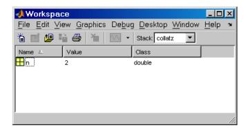
The Value column does not show all details for all variables. To see details, double-click a variable in the Workspace browser. The Array Editor opens, displaying the content for that variable. You can open the Array Editor directly for a variable using openvar.
