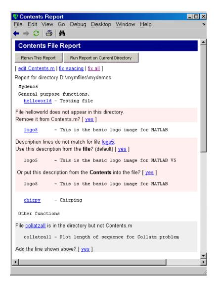
Use the links displayed for each line, or edit the Contents.m file directly, or edit the M-files to make the changes. To make all of the suggested changes at once, click **fix all**. To automatically align the filenames and descriptions in the Contents.m file, click **fix spacing**.
